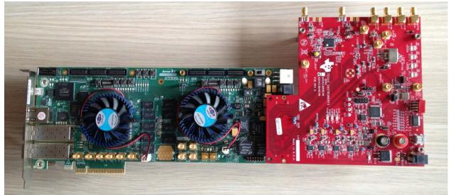
Figure 1 ADS42JB49 Hardware test bed Components
