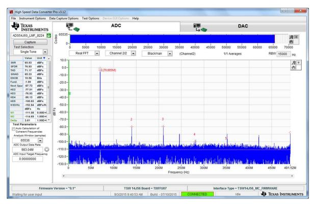
Figure 6. Channel 2 Data Capture Results from Quick Start Procedure
