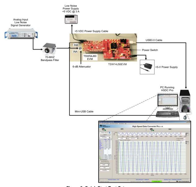
Figure 2. Quick Start Test Setup
