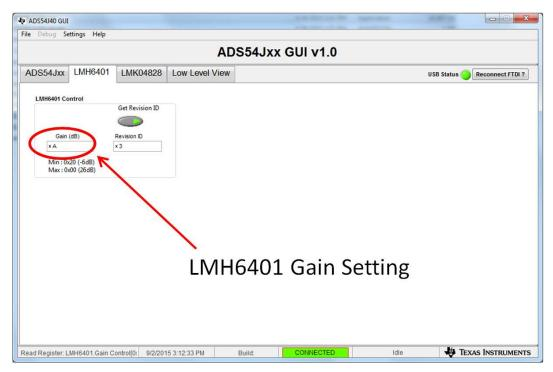
Figure 4. LMH6401 Gain Setting Control
