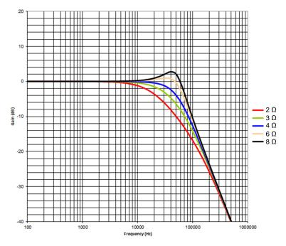
Figure 6. Filter Frequency Response
