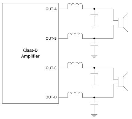
Figure 1. Output Configuration BTL
