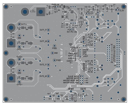
Figure 10. TPA3220 EVM Bottom Composite Assembly
