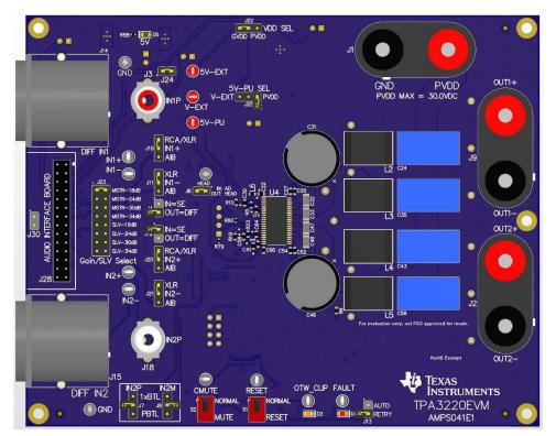
Figure 5. EVM Board With Connectors and Jumpers
