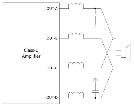
Figure 4. Output Configuration PBTL - 4 Inductors
