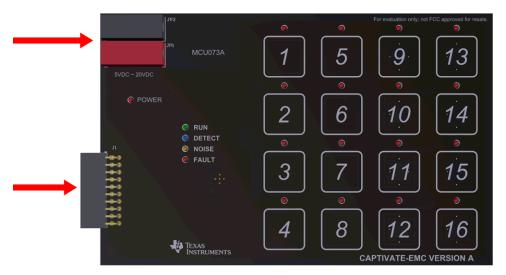
Figure 4. CAPTIVATE-EMC Power Supply Options
