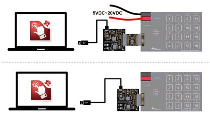
Figure 7. Connection to CapTIvate Design Center
