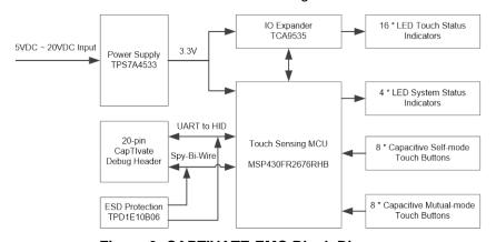
Figure 3. CAPTIVATE-EMC Block Diagram
