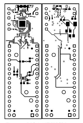
Figure 4-4. DAC53701EVM PCB Layers
