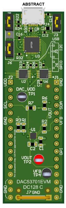
This user's guide describes the characteristics, operation, and use of the DAC53701EVM evaluation module (EVM). This EVM is designed to evaluate the performance of the DAC53701 and DAC43701 (DACx3701) commercial, buffered voltage output DACs in a variety of configurations. Throughout this document, the terms evaluation board, evaluation module, and EVM are synonymous with the DAC53701EVM. This document includes a schematic, printed-circuit board (PCB) layouts, and a complete bill of materials.
