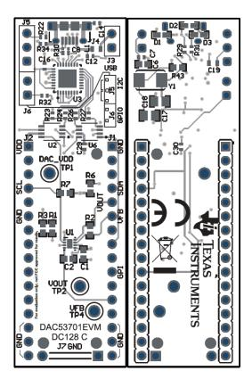
Figure 4-3. DAC53701EVM PCB Components Layout
