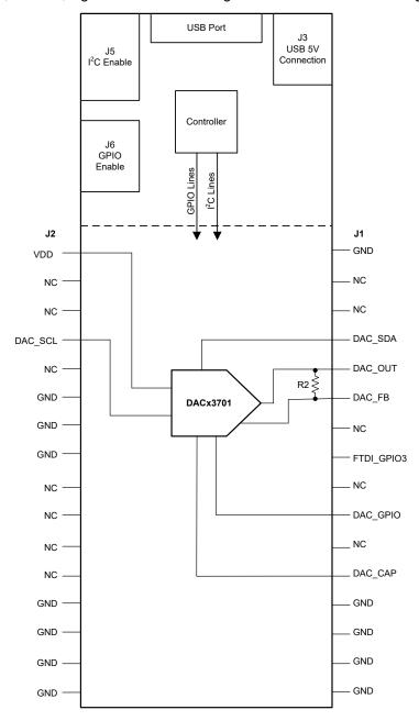
Figure 3-1. DAC53701EVM Hardware Simplified Schematic
