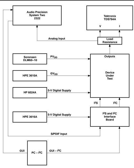
Figure 1. Test Setup Block Diagram
