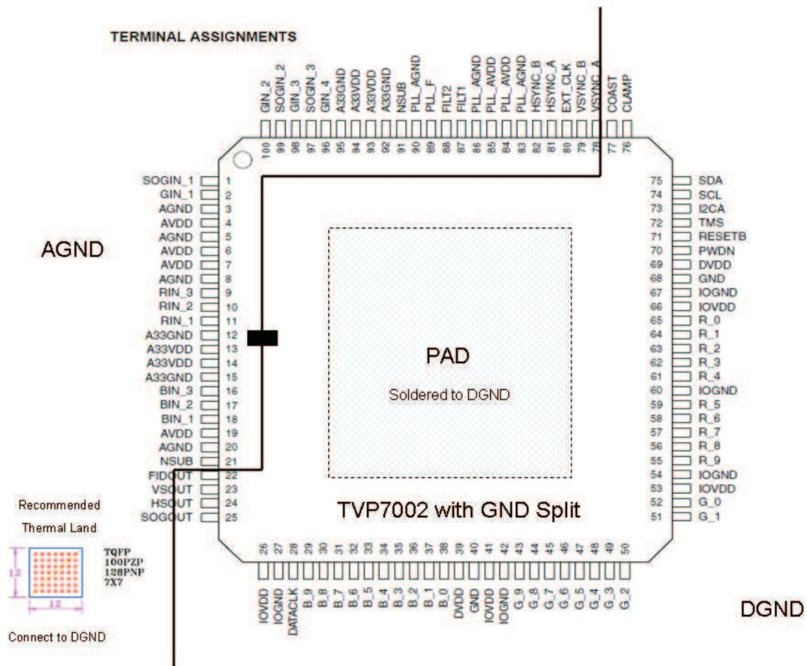
Figure 1. Recommended Split Between Ground Planes
