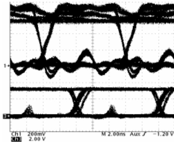
Figure 12. Eye Patterns at Node 4 With 100-Mbps PRBS Into Node 3
