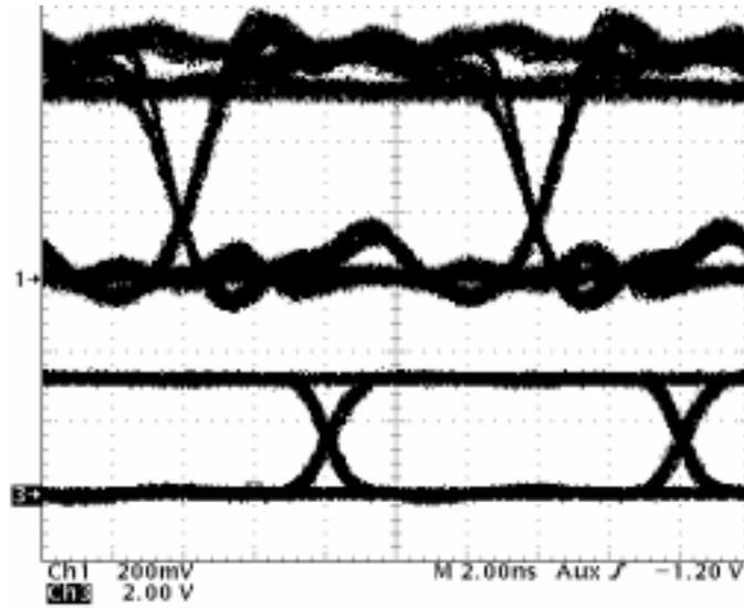
Figure 7. Eye Patterns at Node 3 With 100-Mbps PRBS Into Node 1
