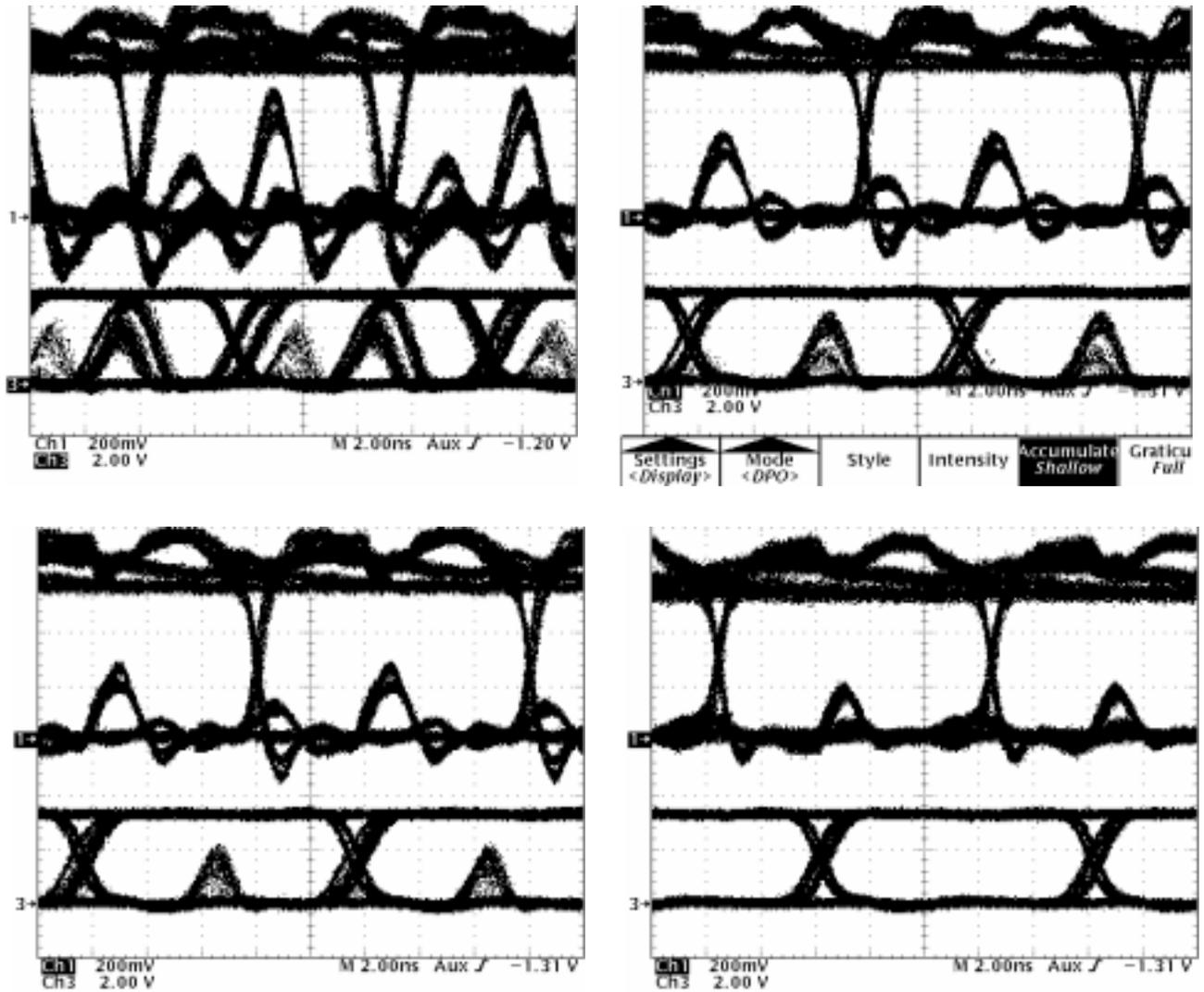
**Figure 14. Eye Patterns Into and Measured at Node 3 as Capacitance Decreased**
