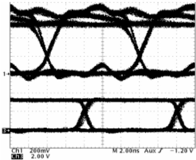
Figure 8. Eye Patterns at Node 4 With 100-Mbps PRBS Into Node 1
