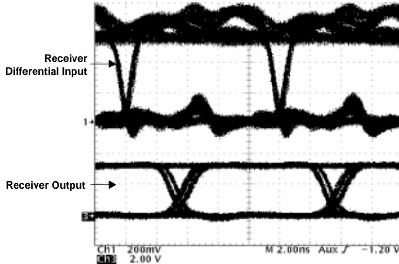
Figure 5. Eye Patterns at Node 1 With 100-Mbps PRBS Into Node 1
