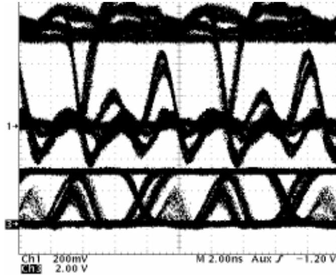
Figure 11. Eye Patterns at Node 3 With 100-Mbps PRBS Into Node 3
