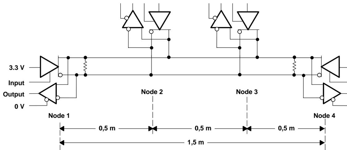
**Figure 4. Test Bus Schematic Diagram**
