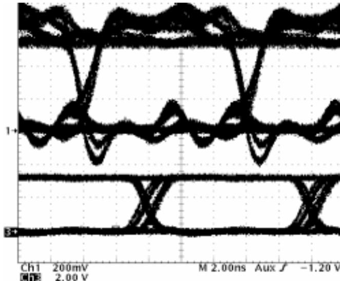
Figure 6. Eye Patterns at Node 2 With 100-Mbps PRBS Into Node 1
