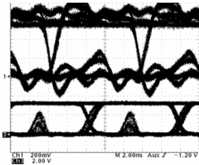
Figure 10. Eye Patterns at Node 2 With 100-Mbps PRBS Into Node 3
