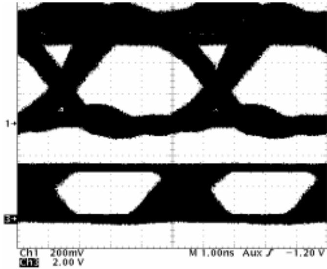
Figure 9. Eye Patterns at Node 4 With 200-Mbps PRBS Into Node 1
