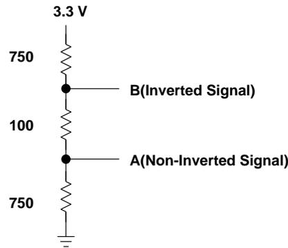
**Figure 15. Termination Modification for Increasing Noise Margin**
