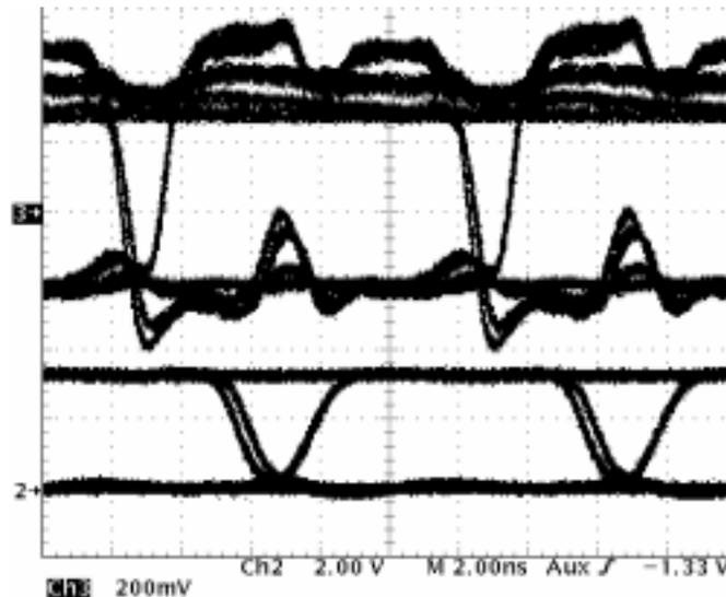
**Figure 16. Eye Patterns at Node 3 With 100-Mbps PRBS Into Node 3 With Modified Terminations**
