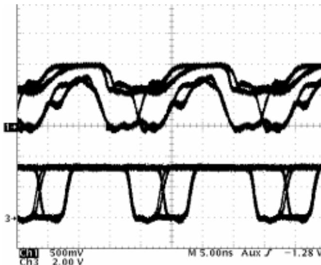
Figure 13. Eye Patterns at Node 4 With PRBS Into Node 3 and Pulse Into Node 1
