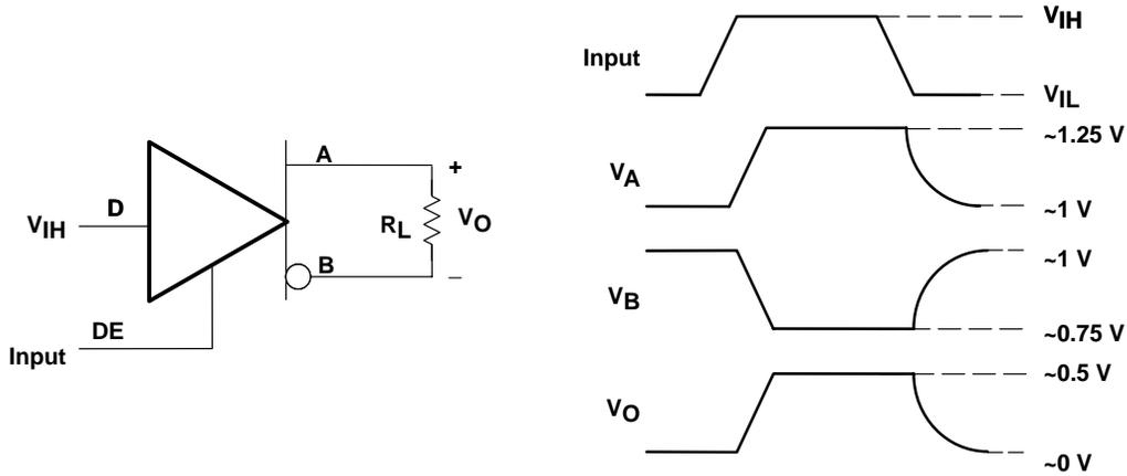
**Figure 2. Wired-OR Operation of M-LVDS Driver**
