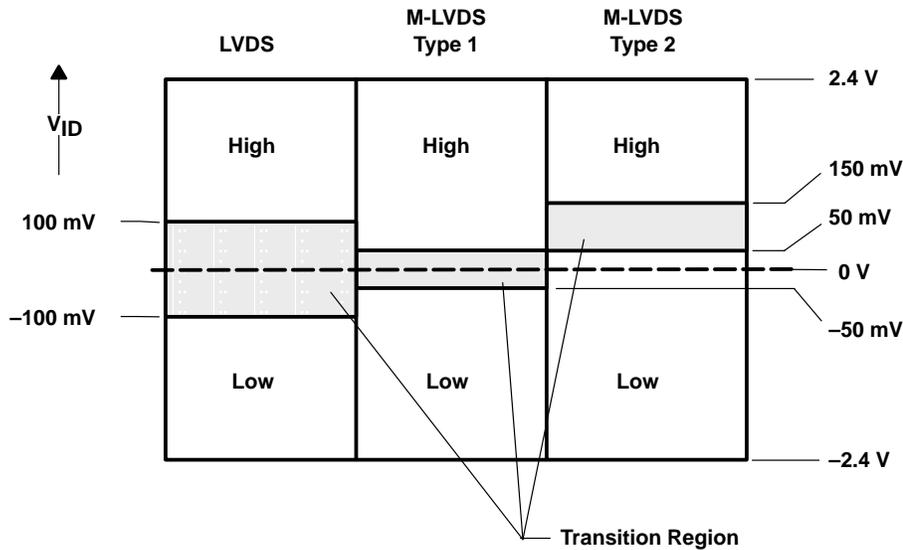
**Figure 3. Differential Input Voltage Threshold Comparison**
