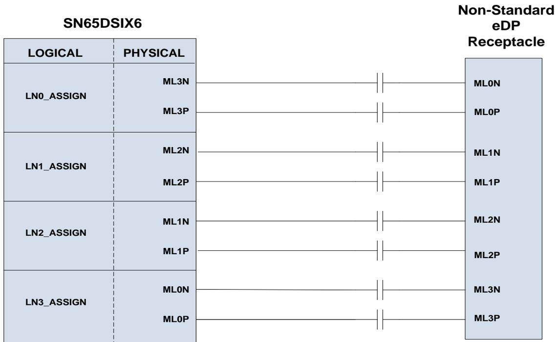
**Figure 3. Custom Lane Assignment Example**
