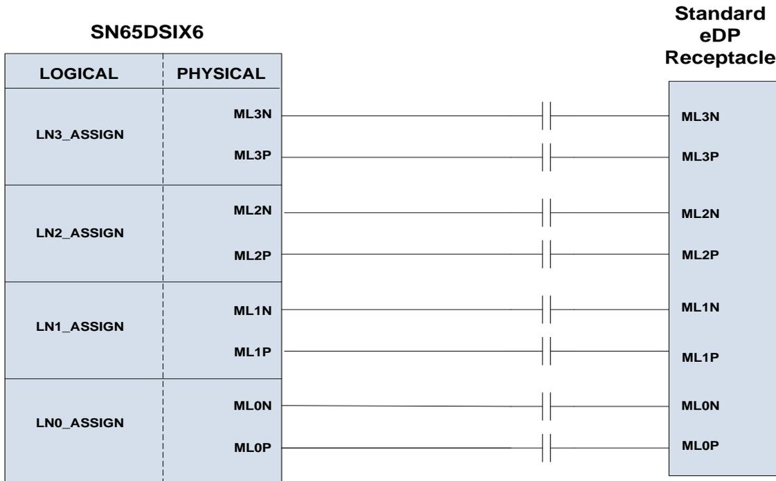
**Figure 2. Default Configuration Lane Assignment Example**
