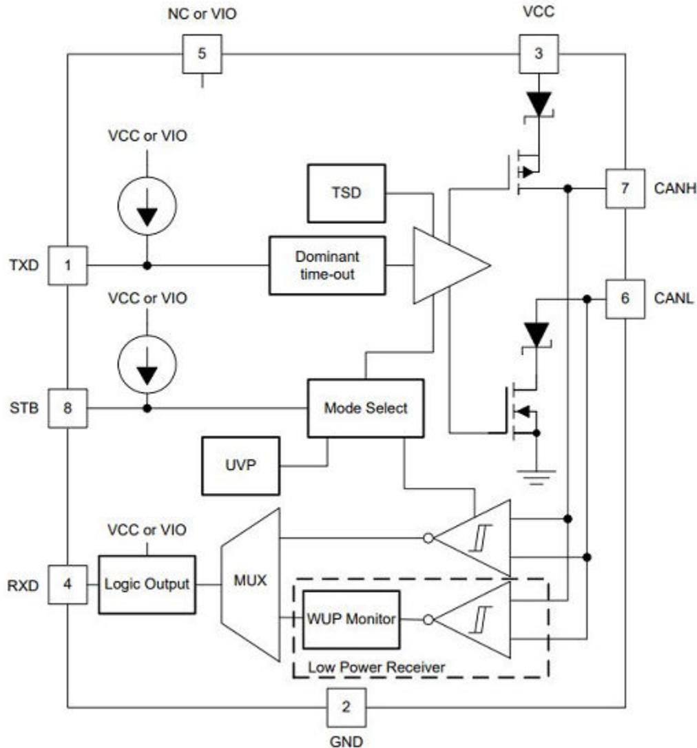
Figure 1-1. TCAN1044-Q1/TCAN1044V-Q1 Functional Block Diagram
