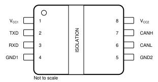
Figure 4-1. Pin Diagram (8-DWV) Package
