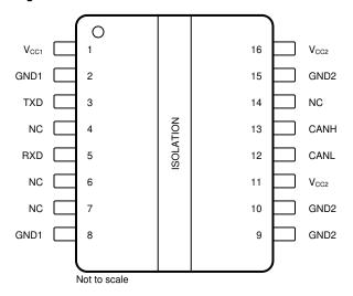
Figure 4-2. Pin Diagram (16-DW Package)
