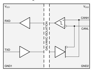
Figure 1-1. Functional Block Diagram
