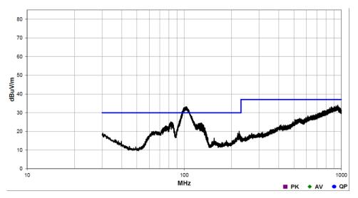
Figure 3-6. Horizontal Radiated Emissions Measurements per CISPR32 Class B for PH9085.011NL with 1m Cable on Isolated GND and no Snubber
