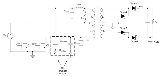
Figure 3-1. Test PCB Configuration with Snubber Circuits
