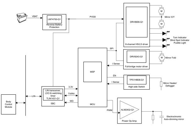
Figure 1. Block Diagram of Typical Side Mirror
