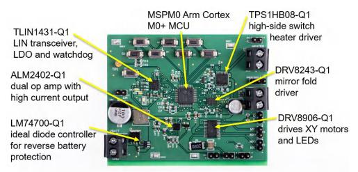
Figure 2. Example Implementation of Side Mirror Module Design
