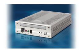
The TI split-chassis PC product demonstration includes a standard PCI Expressenabled desktop PC with a x1 PCI Express cable connector. The I/O hub (shown to the left) is connected to the desktop via a standard PCI Express x1 cable (under definition by the PCI-SIG) and provides 2.5 Gbps of data throughput in both the upstream and downstream directions, providing an aggregate bandwidth of 500MBps.
