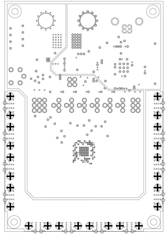
Figure 14. SN65LVCP114 Board Layout: Internal Power (Layer 3 of 6)
