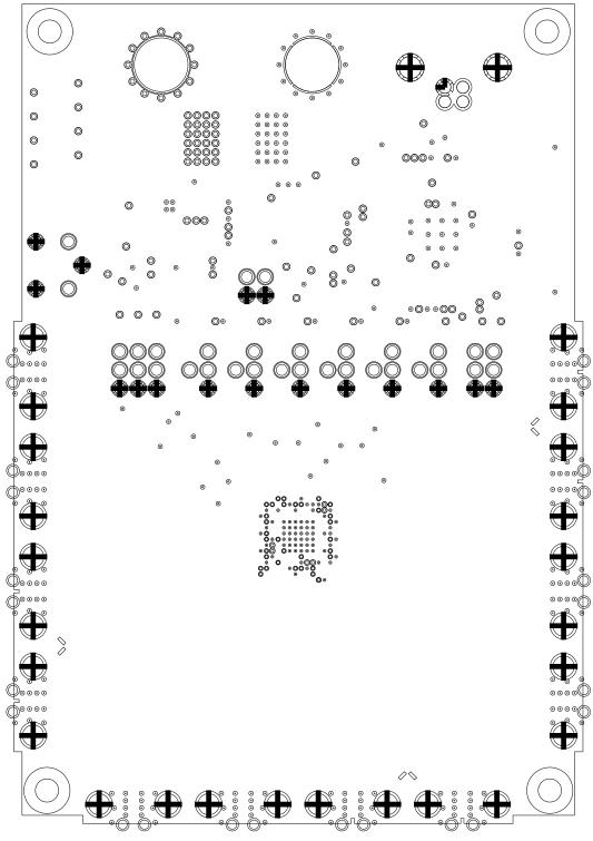
Figure 16. SN65LVCP114 Board Layout: Internal Ground (Layer 5 of 6)
