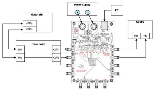
Figure 18. Receive Side Use Case
