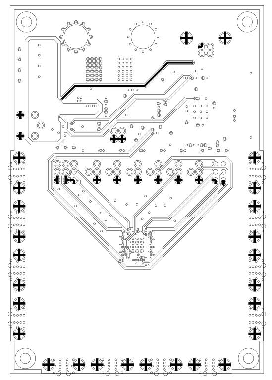
Figure 15. SN65LVCP114 Board Layout: Internal Signal (Layer 4 of 6)
