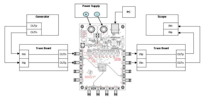
Figure 20. Combined Bus Extension Use Case
