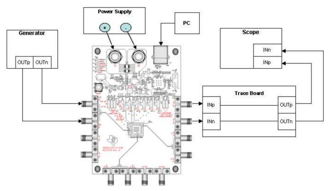
Figure 19. Transmit Side Use Case
