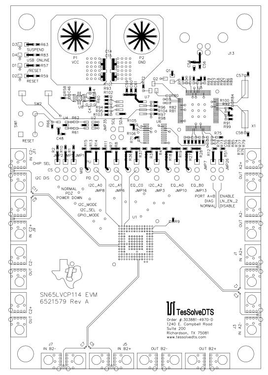
Figure 12. SN65LVCP114 Board Layout: Top Signal (Layer 1 of 6)
