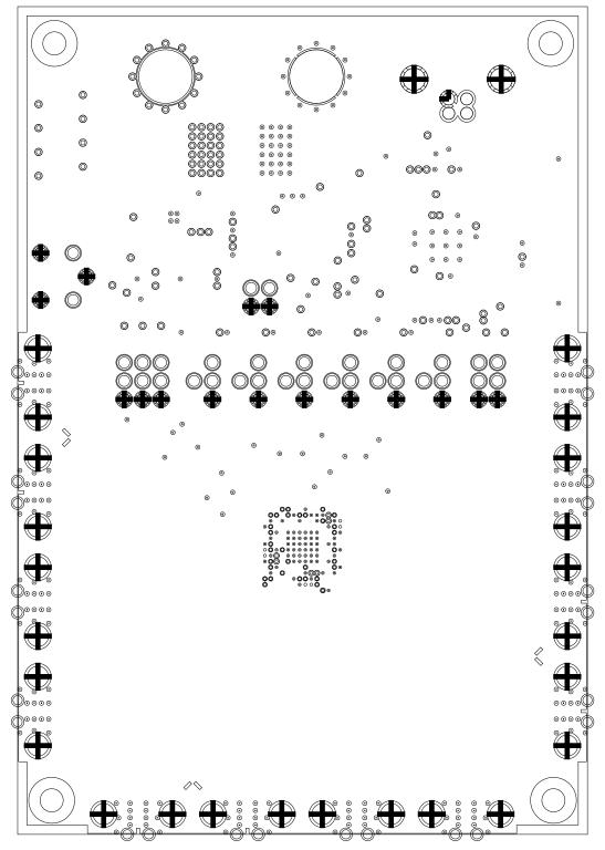
Figure 13. SN65LVCP114 Board Layout: Internal Ground (Layer 2 of 6)
