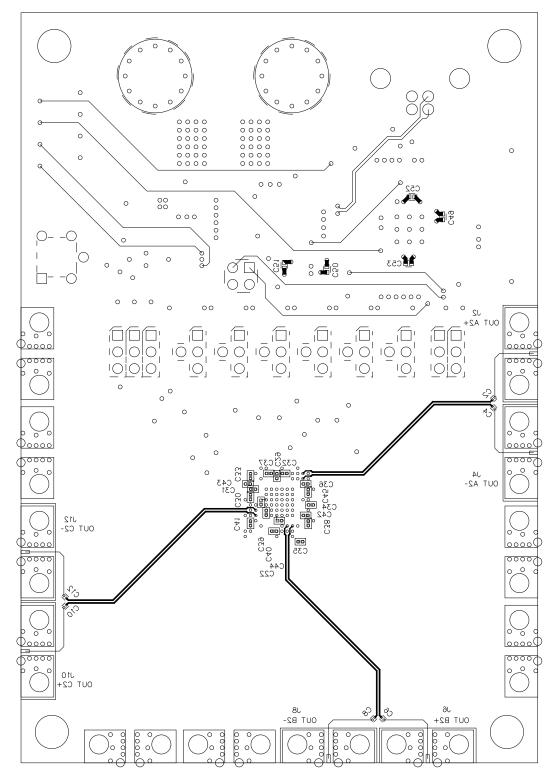
Figure 17. SN65LVCP114 Board Layout: Bottom Signal (Layer 6 of 6)
