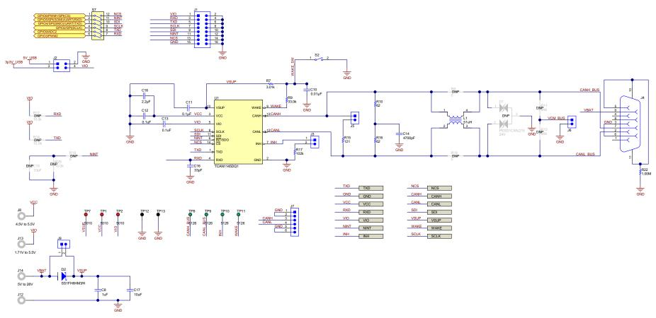
Figure 2. TCAN1145EVM CAN Schematic
