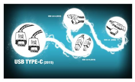
Figure 1: The first USB 2.0 port was made available in 2000. The standard has since evolved to include USB Type-C.
