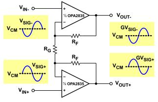
Figure 6. Differential to Differential Amplifier
