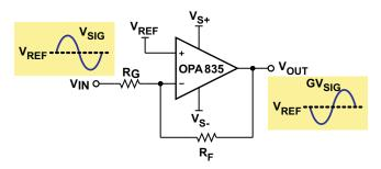
**Figure 2. Inverting Amplifier**
