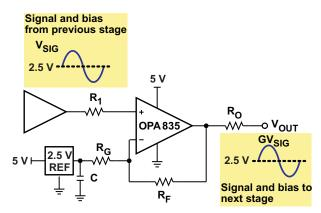
Figure 15. Non-Inverting Single Supply with Reference
