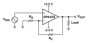
Figure 13. Split Supply Operation
