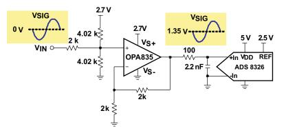
Figure 33. OPA835 and ADS8326 Test Circuit
