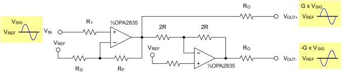
Figure 3. Single Ended to Differential Amplifier
