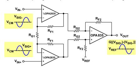
Figure 7. Instrumentation Amplifier
