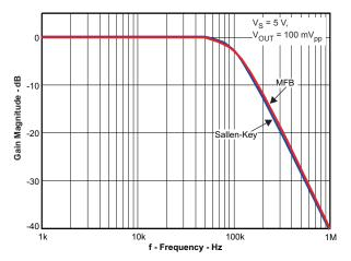
Figure 28. MFB and Sallen-Key 2<sub>nd</sub> Order Low-Pass Butterworth Filter Response
