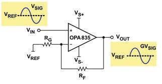
Figure 1. Non-Inverting Amplifier
