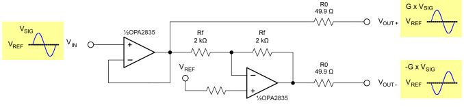
Figure 4. CAT 5 Line Driver with Gain = 2 V/V (6 dB)
