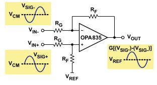
Figure 5. Differential to Single Ended Amplifier
