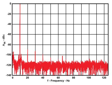
Figure 34. ADS8326 and OPA835 10kHz FFT
