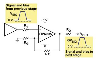
Figure 19. Non-Inverting Single Supply with Pulse
