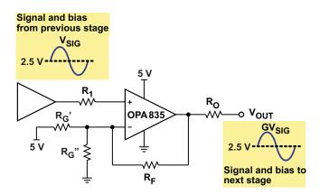
Figure 16. Non-Inverting Single Supply with Resistors
