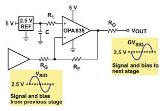
Figure 17. Inverting Single Supply with Reference
