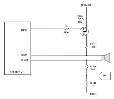
Figure 4-3. Diagnostic Circuit #3 Schematic
