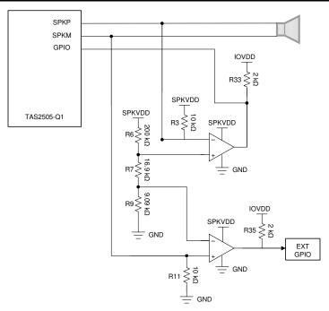
Figure 4-1. Diagnostic Circuit #1 Schematic
