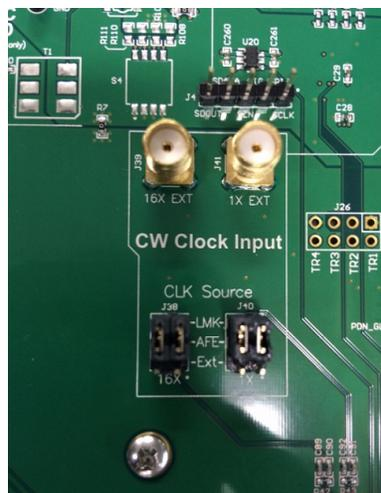
**Figure 8. AFE58xxx8 Default CW Jumper Configuration**
