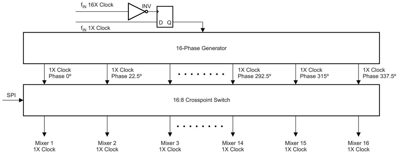
**Figure 2. Phase Generation for 16x Clock Mode**
