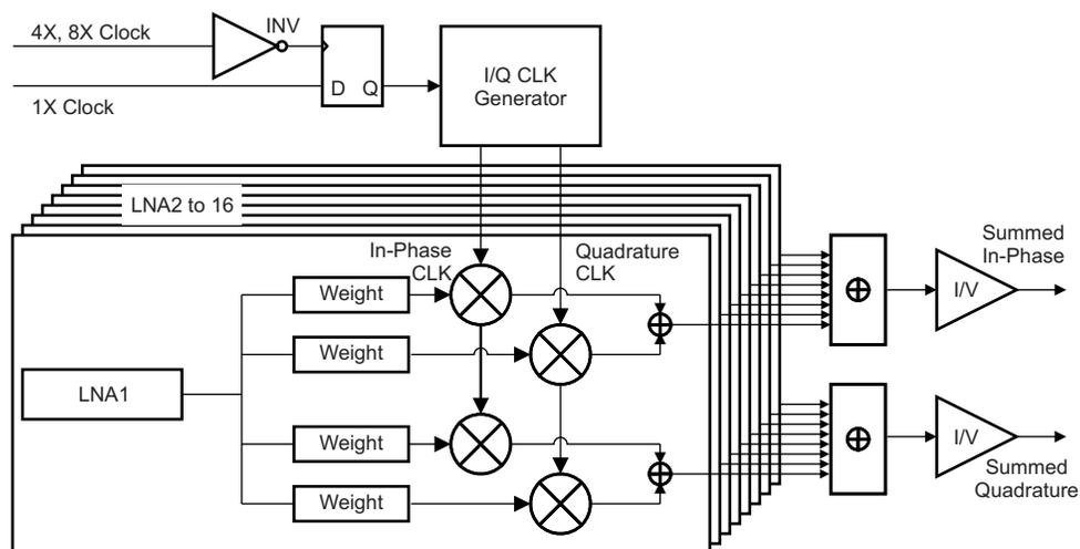
Figure 4. Phase Generation for 8X and 4X Clock Mode
