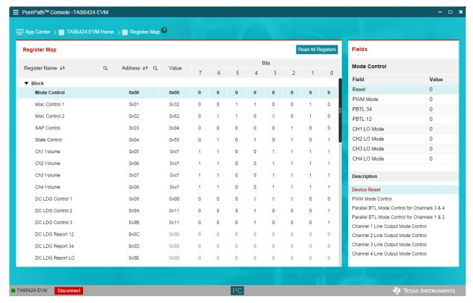
Figure 3-17. Register Map Window - Expanding
