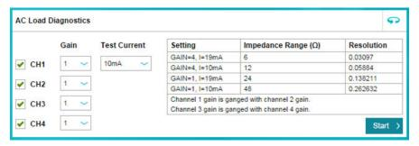
Figure 3-14. AC Load Diagnostics Section
