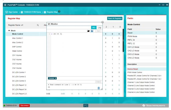
Figure 3-19. I2C Window - Sending I2C Commands
