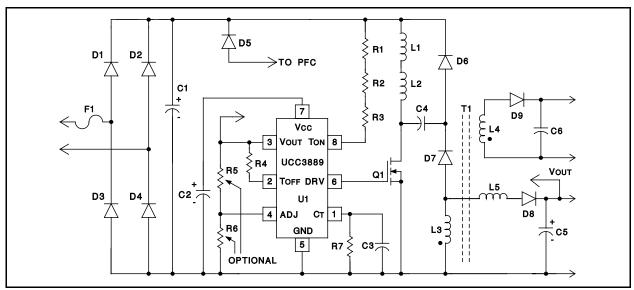
Figure 1. UCC3889 Evaluation Kit Schematic
