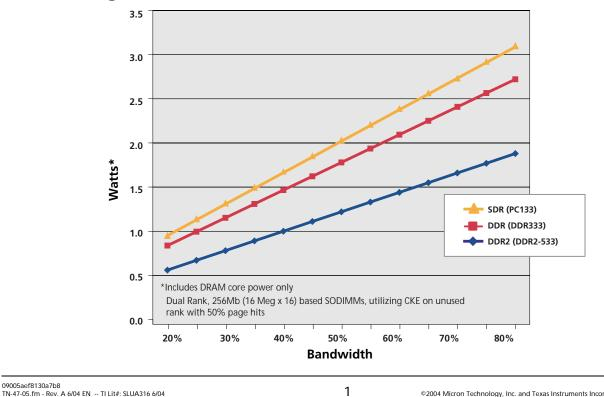
Figure 1: Power Performance Curves on SDR, DDR, and DDR2
