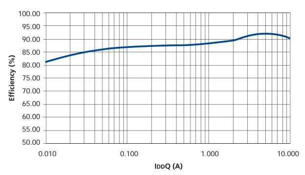
Figure 13: Light Load and Full Load VDD/VDDQ Efficiency
