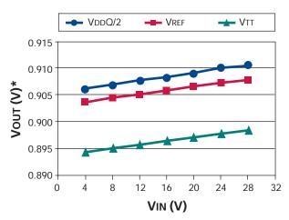
\* Test was performed with a 7A load on VDDQ/2 and a 0.3A load VTT
