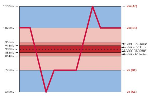
Figure 4: SSTL\_18 Single-Ended Input Logic Levels
