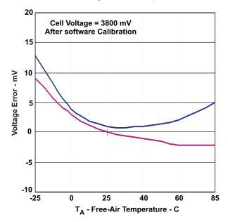
Figure 3. Typical Voltage Error Band After Software Voltage Calibration; Data Measured at 3800 mV Each Cell and Across Temperature
