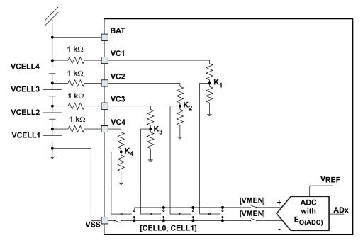
Figure 2. bq3060 Voltage Translation Circuit Diagram
