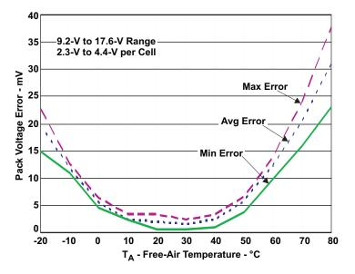
Figure 4. Voltage Error for Post-Calibrated bq803x-Based Devices
