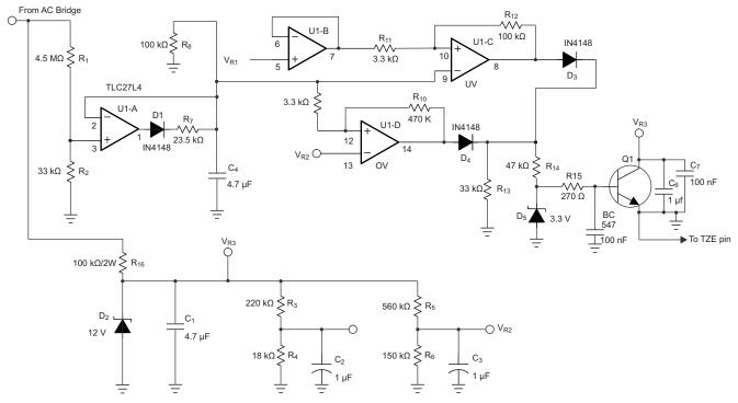
Figure 3. Schematic for Input Undervoltage and Overvoltage Protection
