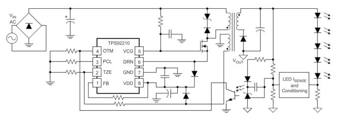
Figure 1. Typical Application Schematic for TPS92210 Based LED Driver
