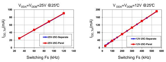
Figure 11. VDD Total Operating Current vs. F<sub>s</sub> at 25°C
