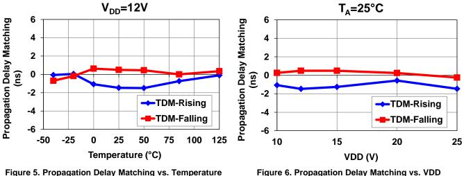
Figure 6. Propagation Delay Matching vs. VDD
