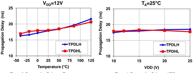
Figure 3. Propagation Delay vs. Temperature
