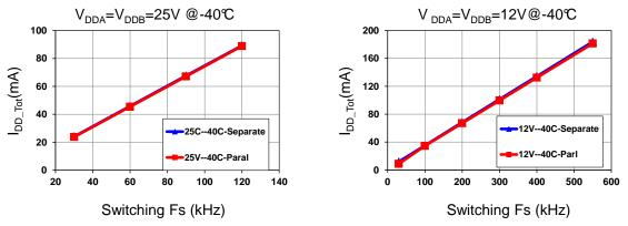
Figure 12. VDD Total Operating Current vs. F<sub>s</sub> at -40°C
