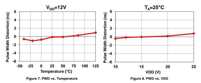
In summary, low propagation delay, low propagation delay matching and low pulse width distortion does position the UCC21520 as the best-in-class gate driver with the best-in-class dynamic response. It is important to note that less than 2-ns propagation delay matching help to parallel the two output channels, double the gate drive strength and increase the versatility of the UCC21520 for a variety of applications.
