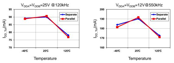
Figure 14. VDD Total Operating Current vs. Temperature at VDD = 12 V and 25 V
