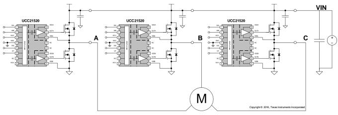
Figure 21. UCC21520 Used in Motor Drives
