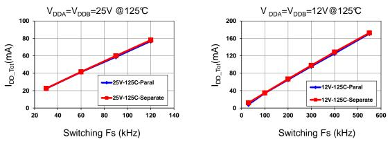
Figure 13. VDD Total Operating Current vs. F<sub>s</sub> at 125°C
