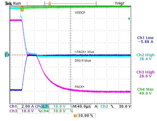
Figure 9. Discharge Disable With Reverse Voltage
