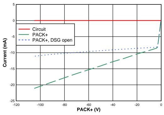
Figure 5. Test Circuit Currents With Reverse Voltage
