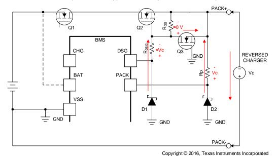
Figure 3. Low Voltage Reverse Voltage Clamp Circuit
