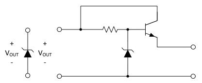
Figure 4. Zener Shunt or Series Pass Regulator to Improve Load Regulation
