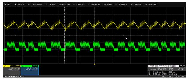
Figure 3. Output Ripple Voltage ( $V_{out}$  = CH1) and Inductor Ripple Current ( $I_{L1}$  = CH4)
