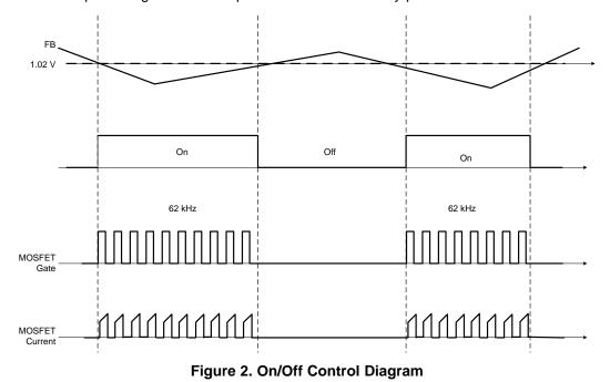
The output inductor ( $L_1$ ) is sized based on internal peak current limit ( $I_{LIMIT}$ ), output current ( $I_{OUT}$ ) and PWM switching frequency of typically 62 kHz. The inductor selected should as close to the calculated value as
