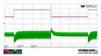
Figure 3. PMP21098 7 A to 14.2 A Transient Response
