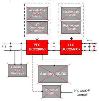
Figure 2. Complete AC-DC Power Supply
