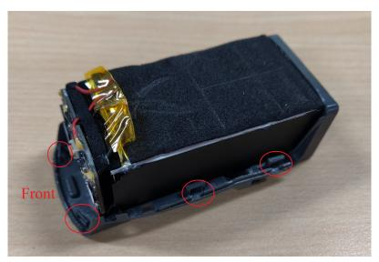
Figure 1. Battery Casing Brackets
