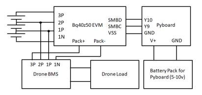
Figure 2. Overview of Wire Connections
