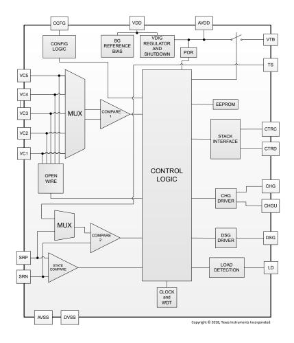
Figure 1-1. Functional Block Diagram
