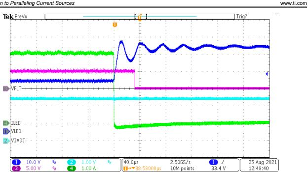
Figure 1-19. Parallel Channels Exposed to Open Circuit Condition Using Modified TPS92519EVM-169
