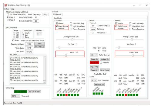
Figure 1-11. Parallel Channels Using Internal PWM Settings Using the GUI
