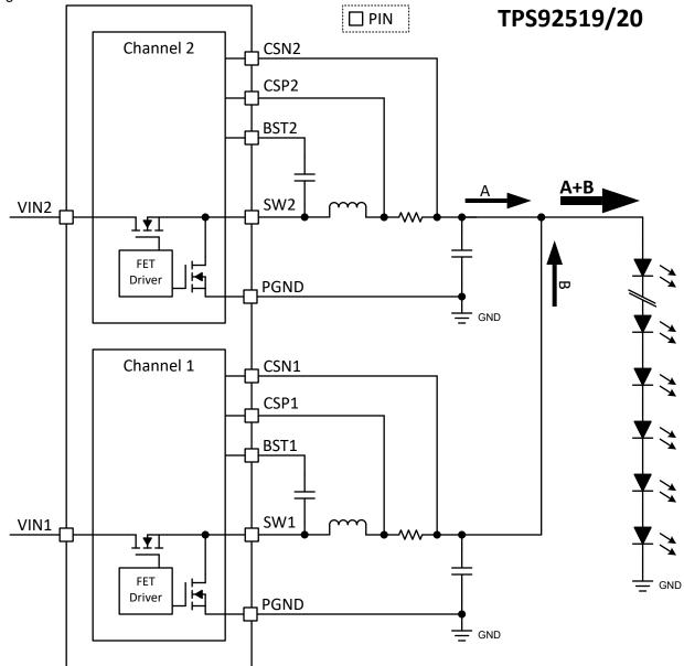
Figure 1-1. Dual Channel LED Driver Connected in Parallel - TPS92519-Q1 and TPS92520-Q1
