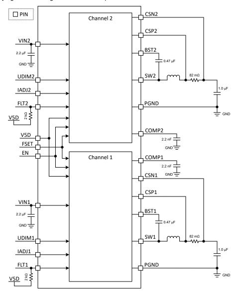
Figure 1-13. High Level Connections for TPS92519-Q1 Dual Synchronous Buck LED Driver
