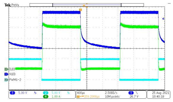
Figure 1-17. Parallel Channels Controlled by PWM Dimming Using Modified TPS92519EVM-169
