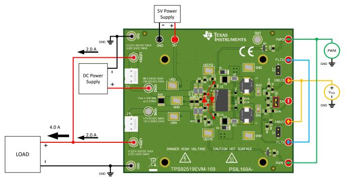
Figure 1-15. Connecting TPS92519EVM-169 for Parallel Operation
