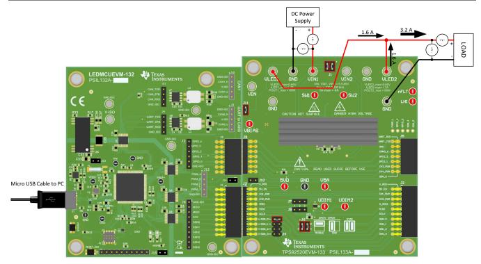
Figure 1-5. Parallel Connection of Outputs Using the TPS92520EVM-133 and LEDMCUEVM-132 Controller
