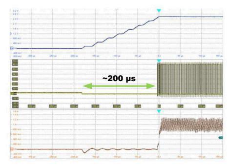
Figure 1-4. Start-up Waveform for a Single Channel
