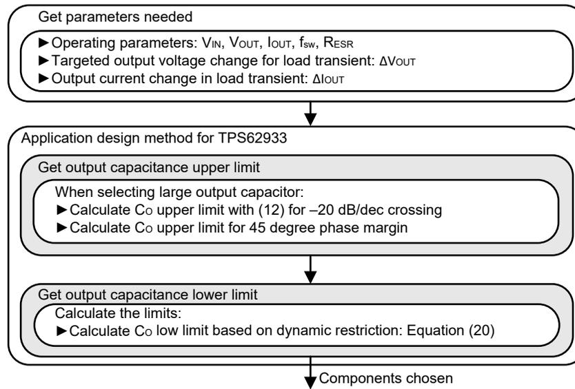
**Figure 5-1. TPS62933 Application Design Flow Chart**
