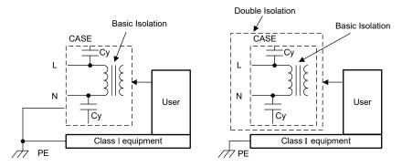
Figure 1-3. Class I and Class II Device
