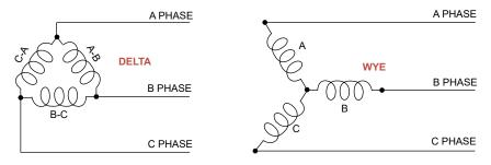
Figure 1-5. Delta and WYE Type of Power Source
