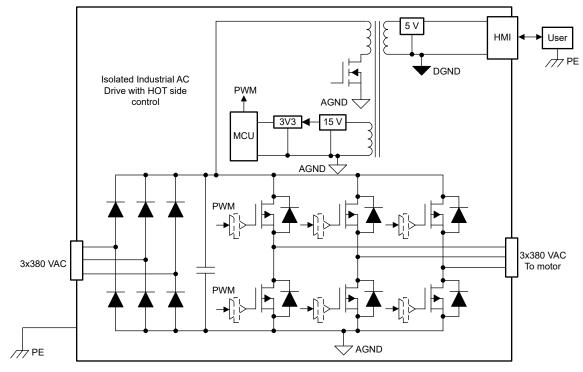
Figure 2-2. Isolated Industrial Motor Drive System Typical Block Diagram
