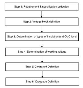
Figure 2-1. Insulation Distance Determining Process
