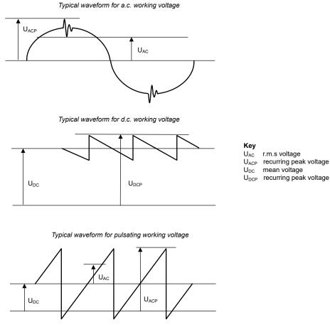
Figure 1-6. Circuit Evaluation for Working Voltage
