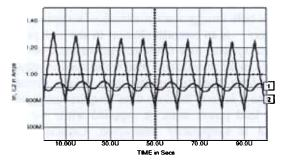
SEPIC Waveforms, Coupled Inductors [1]-IIN, [2]-IL2.
