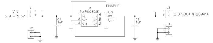
Figure 4. TLV700xxEVM-463 Schematic
