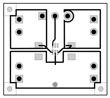
Figure 2. Top Layer Routing
