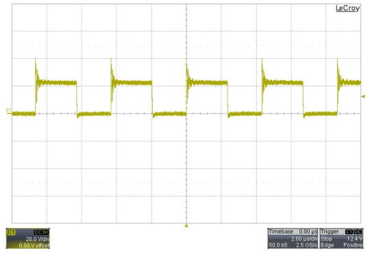
11.3 Q10 Synchronous FET Vds – 400VDC Input, 8.3A Load
