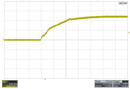
4.4 250VDC Input Startup, 2Ω Load
