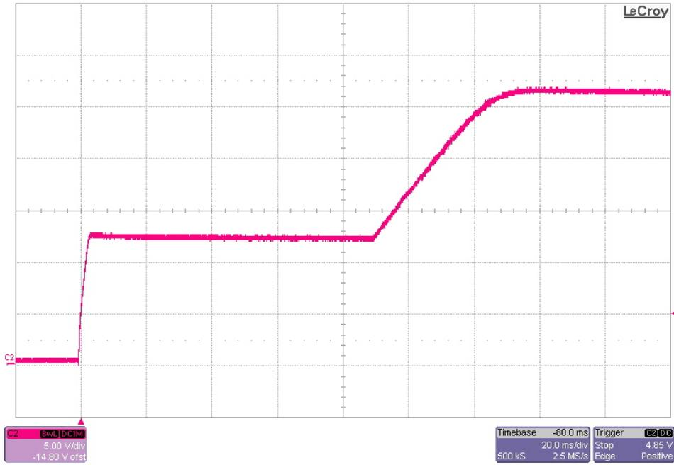
The figure below shows the 26.2V output voltage startup waveform after an input voltage of 12V is applied.  $I_{out} = 10A$ . (5V/DIV, 20ms/DIV)
