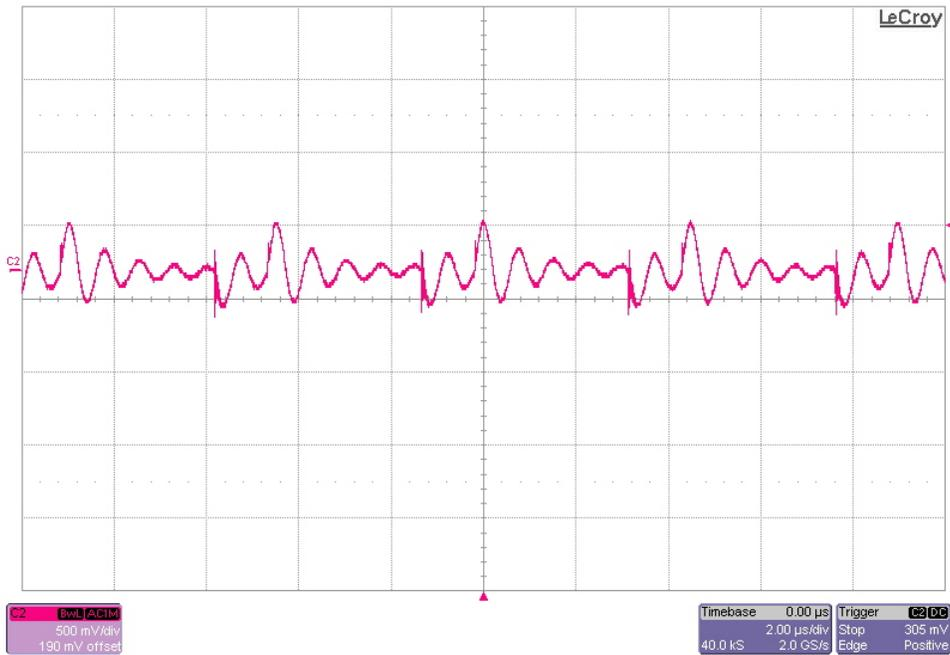
The 26.2V output ripple voltage is shown in the figure below. The image was taken with the output loaded to 10A and the input voltage set to 12Vdc. (500mV/DIV, 2us/DIV)
