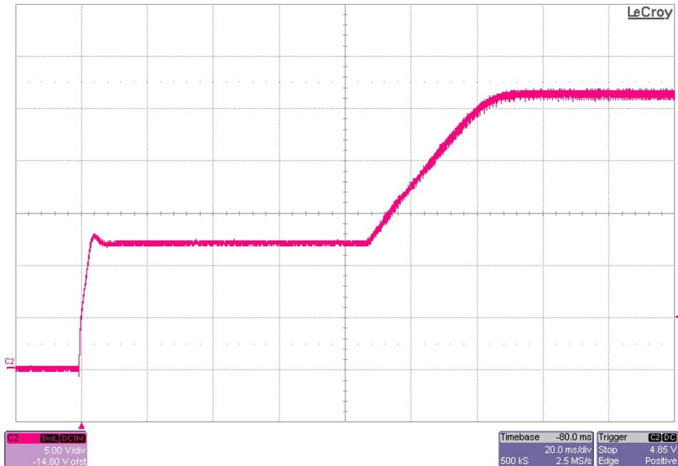
The figure below shows the 26.2V output voltage startup waveform after an input voltage of 25V is applied.  $I_{out} = 6A$ . (5V/DIV, 20ms/DIV)
