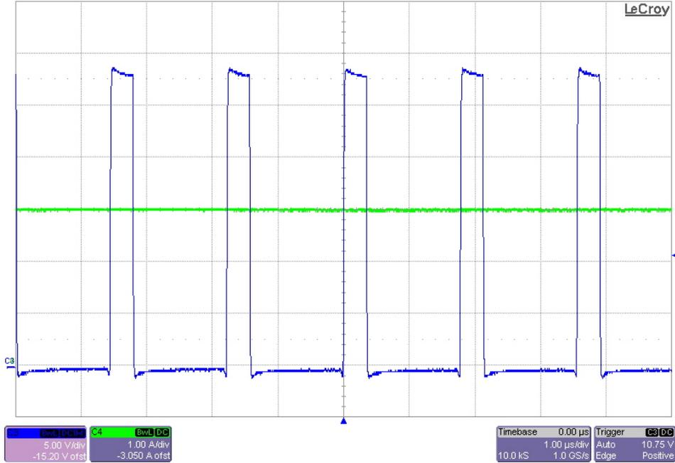
The photo below is of the FET switch node voltage at TP19. The input voltage is 28V and the output cap bank voltage is at 15V while being charged at 3A. A 28.2F/29.7V cap bank was used. (5V/DIV, 1A/DIV, 1us/DIV)
