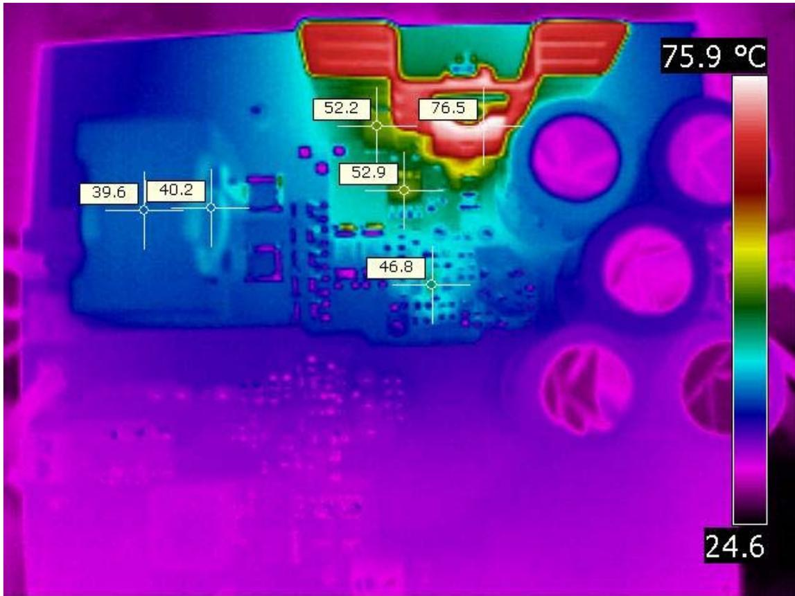
The photo below shows the board temperature when operated at 12V input and 26.2V @ 5A output.
