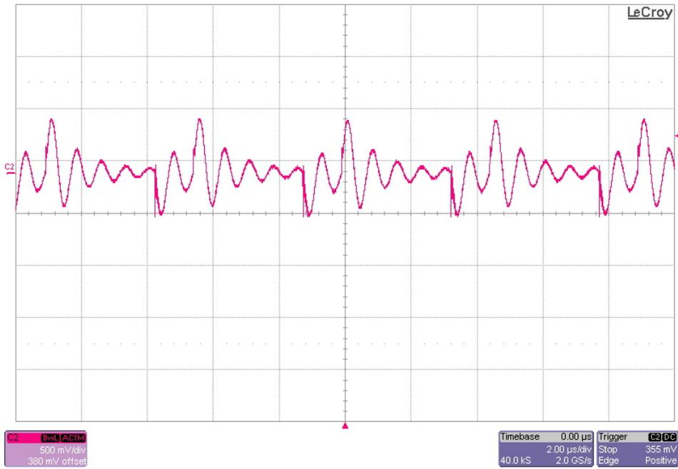
The 26.2V output ripple voltage is shown in the figure below. The image was taken with the output loaded to 6A and the input voltage set to 20Vdc. (500mV/DIV, 2us/DIV)
