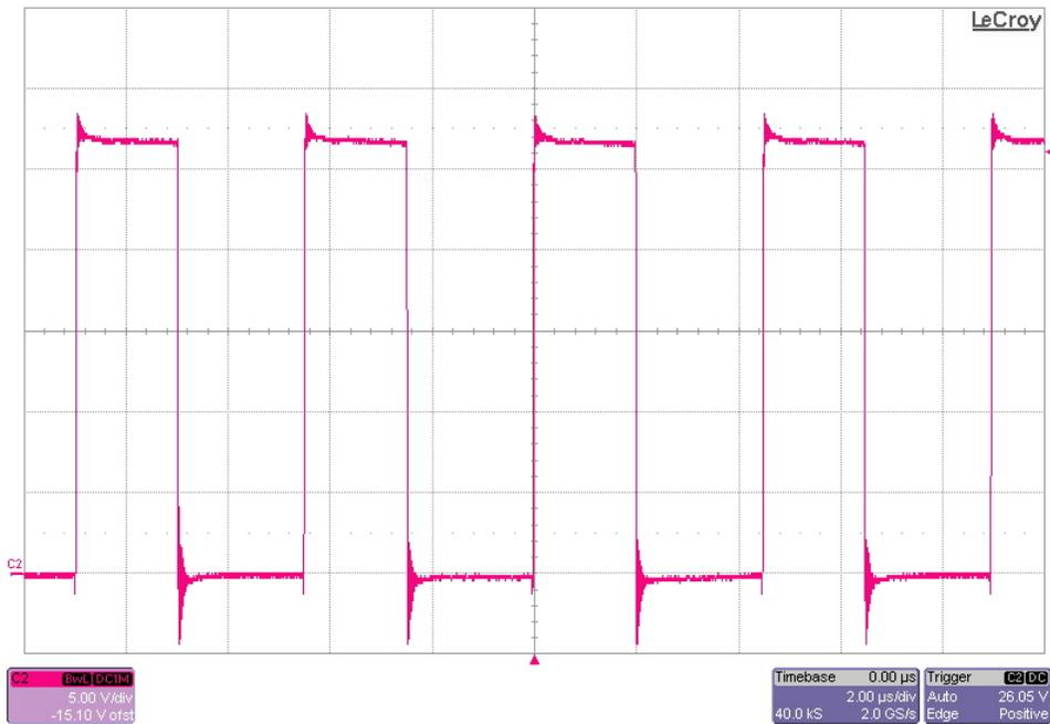
The photo below is of the FET switch node voltage at TP7. The input voltage is 26V and the output is loaded to 10A. (5V/DIV, 2us/DIV)
