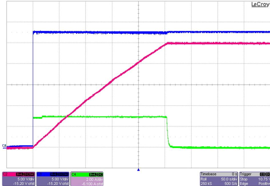
The photo below shows the supercap bank being discharged by the boost converter. A charged supercap (25.2V) is supplying power to the TPS40210 boost converter and loaded to 10A ( $V_o = 26V$ ) until it shuts off. A 28.2F/29.7V cap bank was used. (5V/DIV, 5A/DIV, 5s/DIV)
