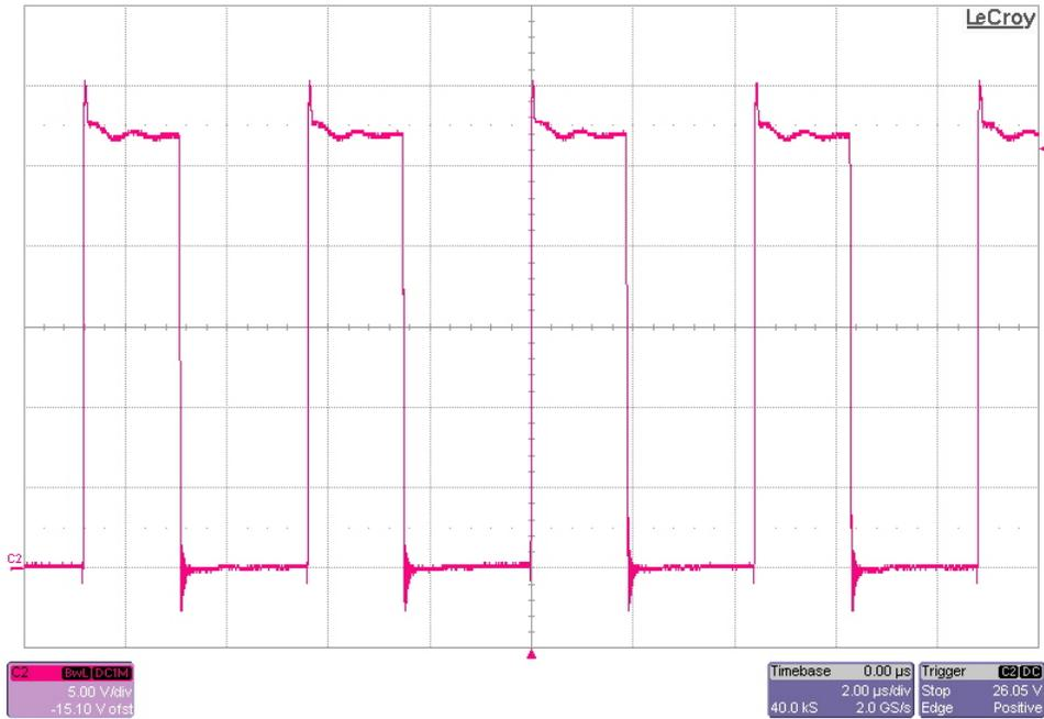
The photo below is of the FET switch node voltage at TP7. The input voltage is 12V and the output is loaded to 1A. (5V/DIV, 2us/DIV)
