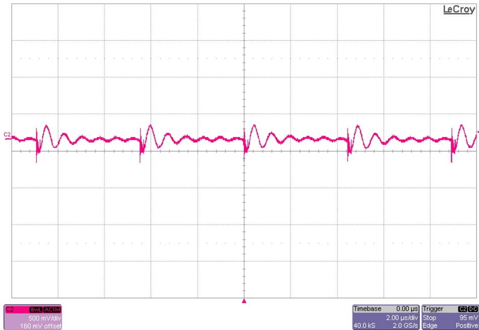
The 26.2V output ripple voltage is shown in the figure below. The image was taken with the output loaded to 10A and the input voltage set to 20Vdc. (500mV/DIV, 2us/DIV)
