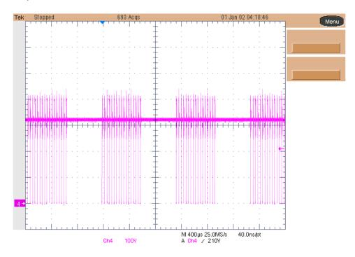
Ch4: Drain voltage (100V/div, 1msec/div, No BWL). Vin = 320Vdc, No Load
