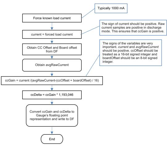
Figure 3-6. Current Calibration Flow
