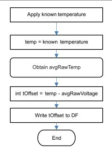
Figure 3-7. Temperature Calibration Flow
