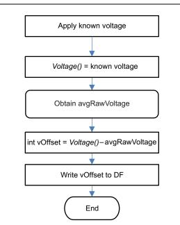
Figure 3-2. Voltage Calibration Flow
