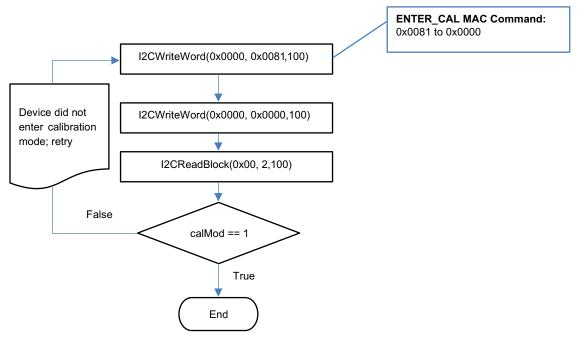
Figure 3-1. Enter CALIBRATION Mode Flow
