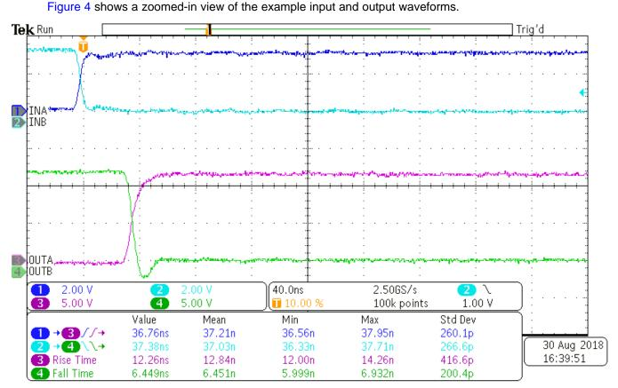
Figure 4. Example Input and Output Waveforms, Zoom In (Inputs: CH1 and CH2, Outputs: CH3 and CH4)
