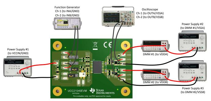
Figure 2. Bench Setup Diagram and Configuration
