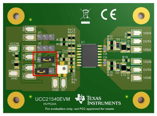
Figure 1. Jumpers Installation Position
