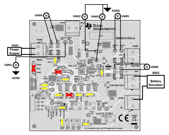
Figure 1. BQ25886 Charge Mode Test Setup
