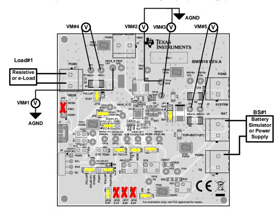
Figure 3. BQ25886 OTG Mode Test Setup
