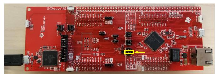
Figure 26. LaunchPad Connection for Programming
