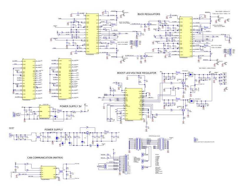
Figure 8. TPS92520EVM-074 Schematic
