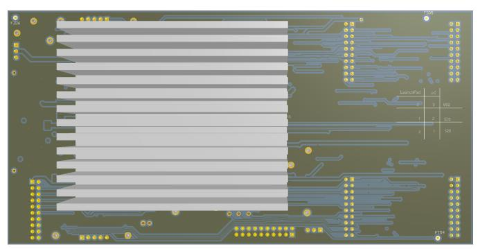
Figure 13. TPS92520EVM-074 Bottom Layer (Bottom View)
