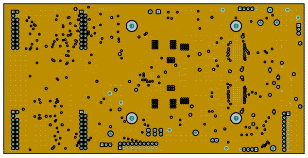
Figure 11. TPS92520EVM-074 Inner Layer (Ground Plane)
