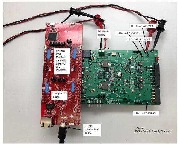
Figure 33. LaunchPad Connection to the TPS92520EVM-074
