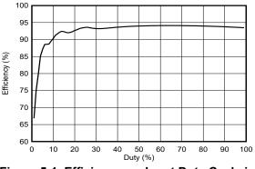
Figure 5-1. Efficiency vs. Input Duty Cycle in Analog Dimming Mode
