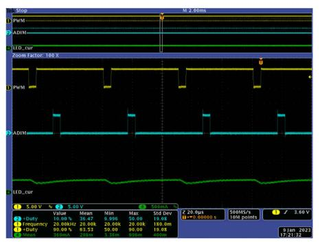
Figure 5-15. Waveforms at 10% Duty Cycle ADIM/HD and 90% Duty Cycle PWM/EN
