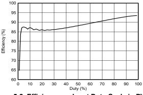
Figure 5-2. Efficiency vs. Input Duty Cycle in PWM Dimming Mode
