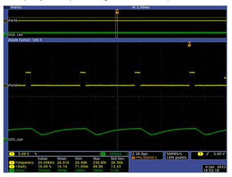
Figure 5-11. Waveforms at 10% Duty Cycle, 20 kHz Hybrid Dimming
