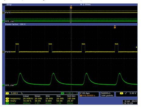
Figure 5-7. Waveforms at 10% Duty Cycle, 20 kHz PWM Dimming
