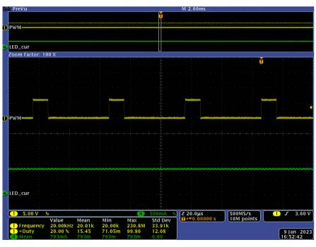
Figure 5-12. Waveforms at 20% Duty Cycle, 20 kHz Hybrid Dimming
