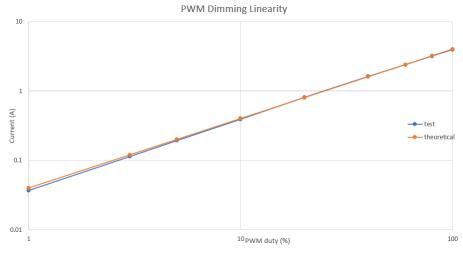
Figure 5-10. PWM Dimming Linearity
