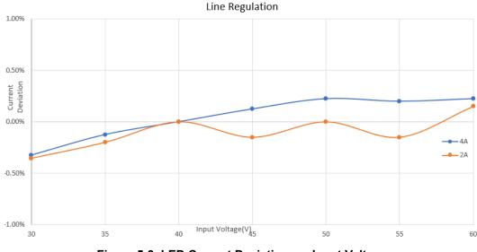
Figure 5-3. LED Current Deviation vs. Input Voltage
