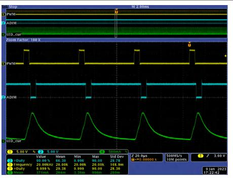
Figure 5-16. Waveforms at 90% Duty Cycle ADIM/HD and 10% Duty Cycle PWM/EN
