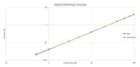
Figure 5-13. Hybrid Dimming Linearity
