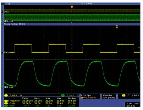
Figure 5-8. Waveforms at 50% Duty Cycle, 20 kHz PWM Dimming
