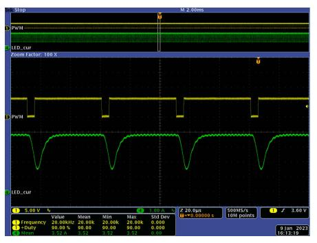
Figure 5-9. Waveforms at 90% Duty Cycle, 20 kHz PWM Dimming
