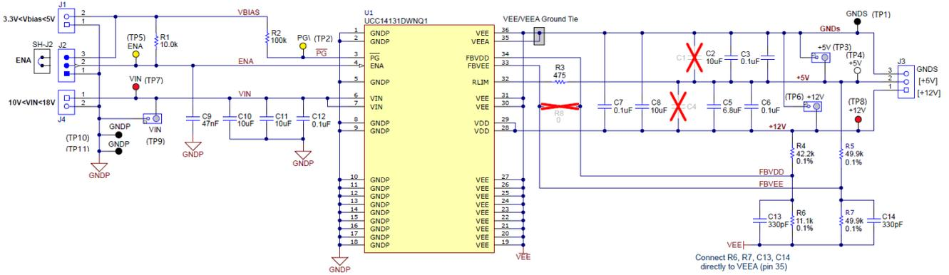
Figure 3-1. UCC14131EVM-070 Schematic Diagram
