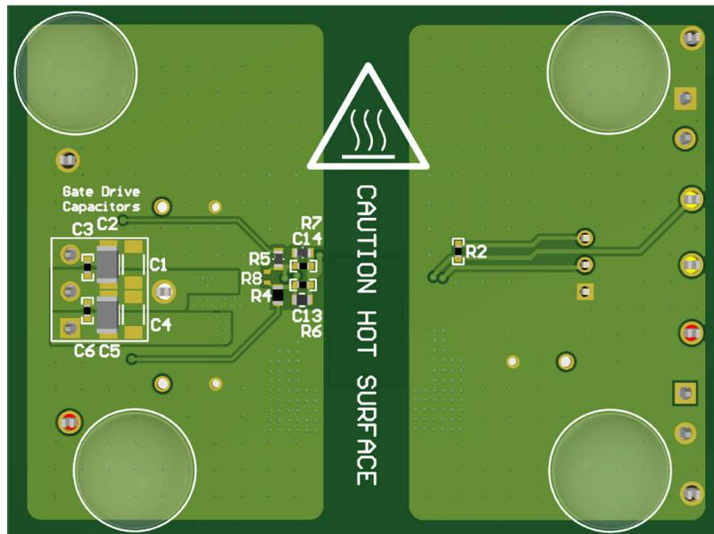
Figure 6-2. UCC14131EVM-070, Fully Assembled 3D Bottom View
