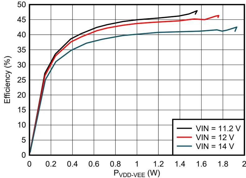
Figure 5-1. Measured Efficiency, VDD-VEE = 12-V Loading Only
