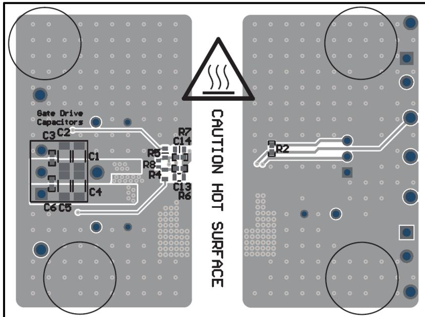
Figure 6-7. UCC14131EVM-070, PCB Bottom Layer, Assembly (mirrored view)
