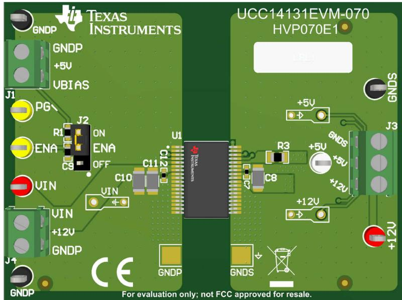
Figure 6-1. UCC14131EVM-070, Fully Assembled 3D Top View
