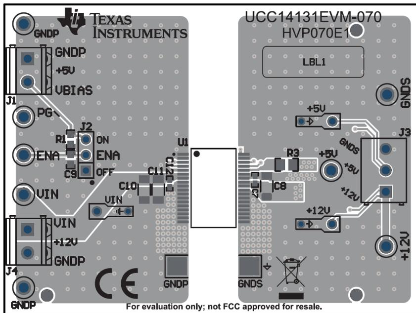
Figure 6-4. UCC14131EVM-070, PCB Top Layer, Assembly
