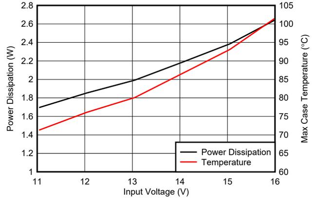
Figure 5-24. Power Dissipation and Case Temperature vs Input Voltage,  $T_A=24.6^\circ\text{C}$ ,  $1.54\text{ W}$
