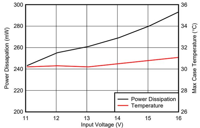
Figure 5-26. Power Dissipation and Case Temperature vs Input Voltage,  $T_A=23.9^\circ\text{C}$ ,  $0\text{ W}$
