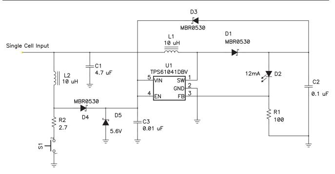
Figure 3. Single Cell Operation With Push-Button Startup
