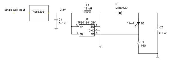
Figure 1. Single Cell Operation With Intermediate Voltage Conversion
