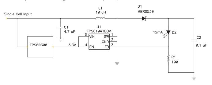
Figure 2. Single Cell Operation With Auxiliary Bias Voltage
