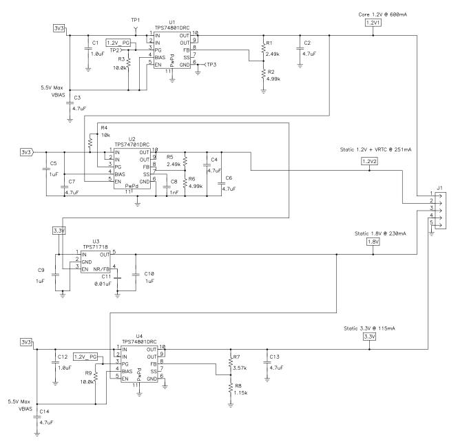
Figure 1. PMP4980 Reference Design Schematic
