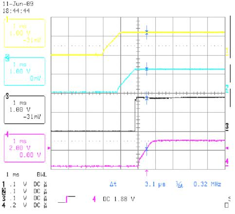
Figure 3. Sequencing in Start-Up Waveform
