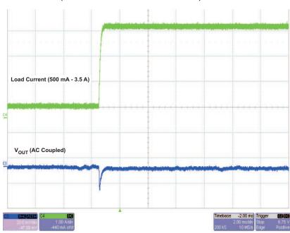
Channel 3 : Vout (AC coupled) Channel 4 : Load current ( Varies between 500mA to 3.5A )
