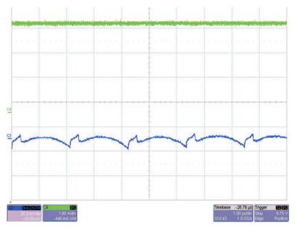
Figure 4. Output Ripple Waveform
