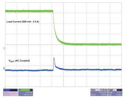
Figure 3. Output Response to Load Transients
