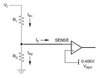
Figure 2. Sense pin for the TPS3808G01
