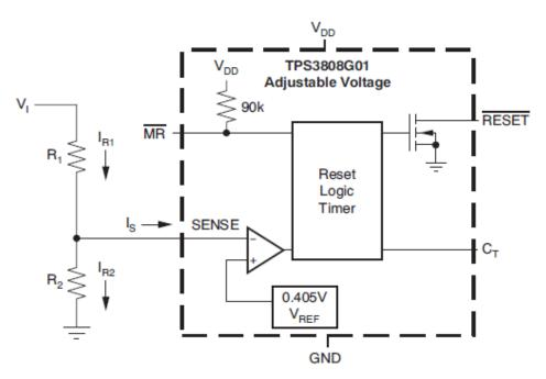
Figure 1. Functional Block Diagram of the TPS3808G01
