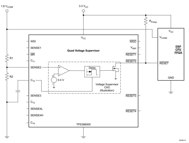
Figure 3. SVS Circuit for Monitoring a Supply Voltage for a CPU Core
