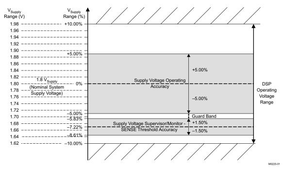
Figure 2. Illustration Depicting a Supply Voltage, the Relative SVS Reset Threshold, and Respective Accuracies Within the Required System Operating Voltage Range
