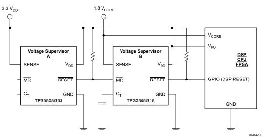
Figure 1. Typical Supply Voltage Supervisor Configuration for Protecting a DSP
